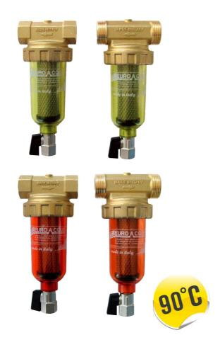
NANOFILTRO 1/2" - 3/4"/1": It is the smallest self-cleaning filter. The solid particles are filtered by the stainless steel cartridge, then flushed out easily by opening the drain valve.
